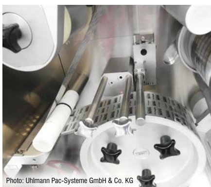
Foreign body detection in medical technology MDS sensor recognizes foreign bodies in blister machines during the tablet packaging process.
