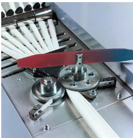
Inline yarn thickness measurement
