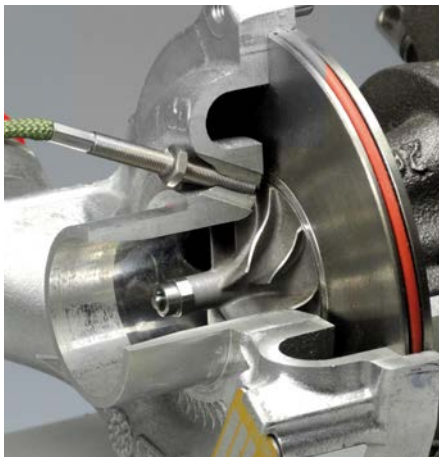
Rotational speed measurement of turbochargers
