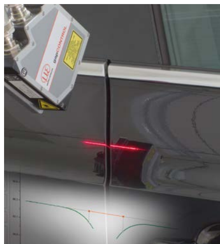
Gap and flushness measurement on bodywork parts
