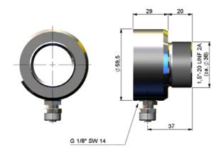
Fig. 3.2: Air purge collar [TM-AP-CX]; Hose connection: 6x8 mm
