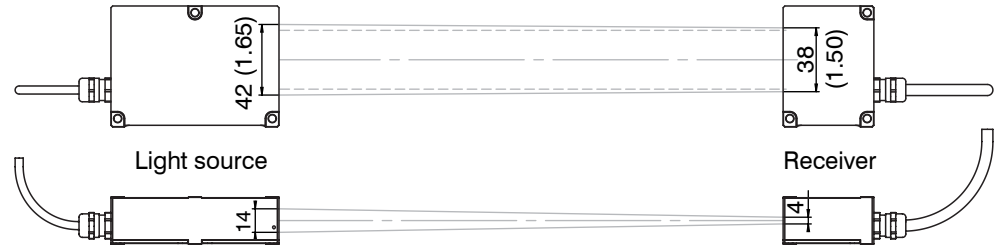
Fig. 47 Free space for the light beam between light source and receiver
