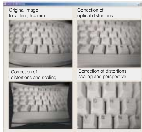
Correction of optical and perspective distortions (wide angle objective)
