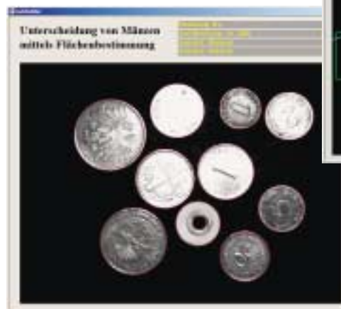
Area and region analysis (coin inspection)
