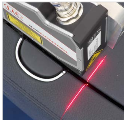
Distance measurement at the center console
