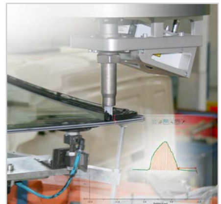
Inspection of the adhesive beading
