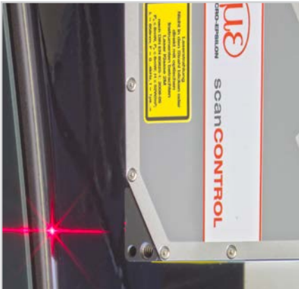
Gap measurement on car bodies
