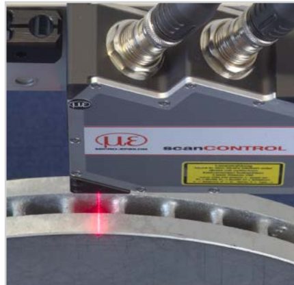
Profile measurement of the brake disc
