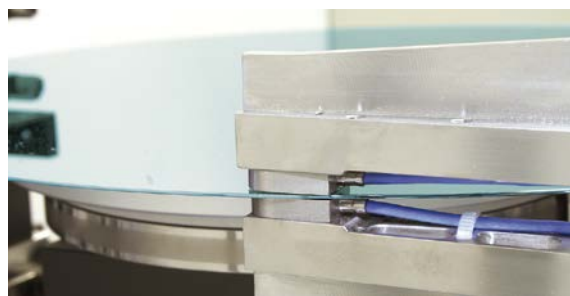
Wafer thickness measurement with two capacitive sensors
