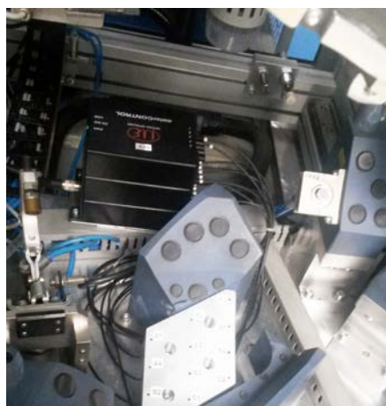
Color and intensity tests of vehicle lights.
