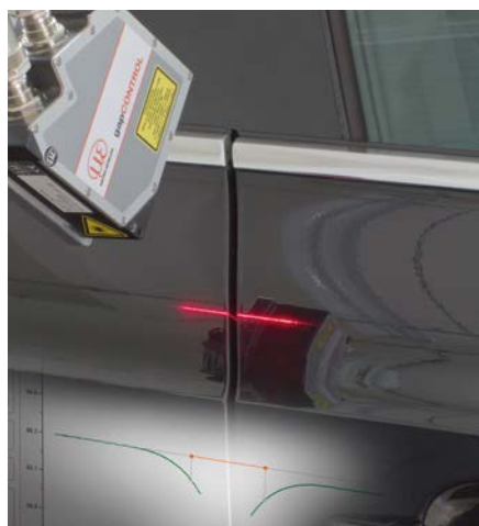
Gap and flushness measurement on bodywork parts
