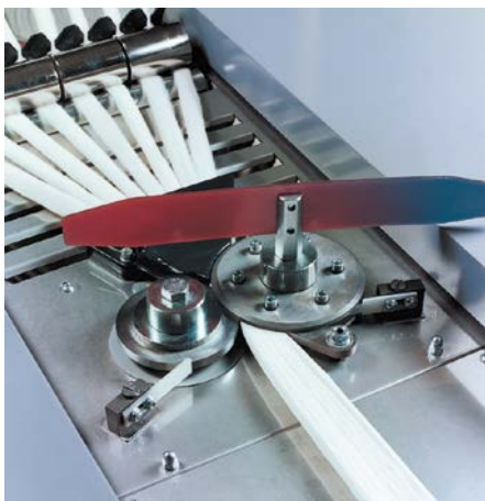
Inline yarn thickness measurement
