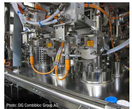
Valve lift measurement in the food industry The sealed stainless steel housings of the MDS-45-Mxx series are ideal for the food industry.
